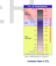
$CO_2$  ventilation control is a real time air balancing system that ensures the right amount of ventilation is provided at all parts of your building to ensure acceptable indoor air quality. This approach called automatic ventilation control.
