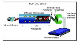
Fig.3. Non-dispersive infrared detection (NDIR) CO<sub>2</sub>
